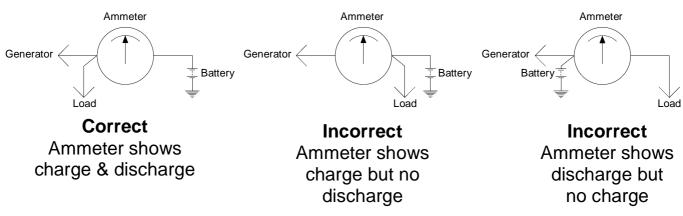
With the engine stopped, and lights turned on, ammeter shows correct discharge. When the engine is running at charging speed with no lights the ammeter shows an incorrect discharge, when the lights are turned on the ammeter shows an even greater discharge, further increase in engine speed dims the lights slightly.
